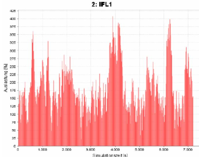
**Figure 10: Time dependent utilization for an IFL-processor**
