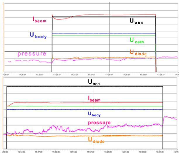
Figure 4. Operation parameters for the 180 s, 950 kW. (top) and the 1893 s, 540 kW pulse (bottom).
