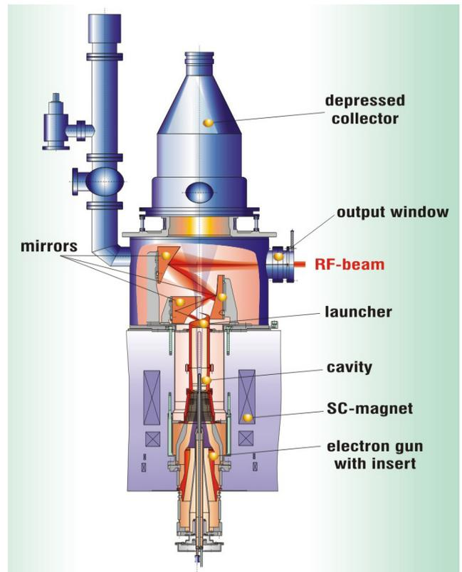
Figure 1. View of the 170 GHz pre-prototype gyrotron.
