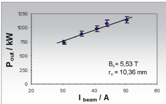
Figure 2. Dependence of output power on electron.
