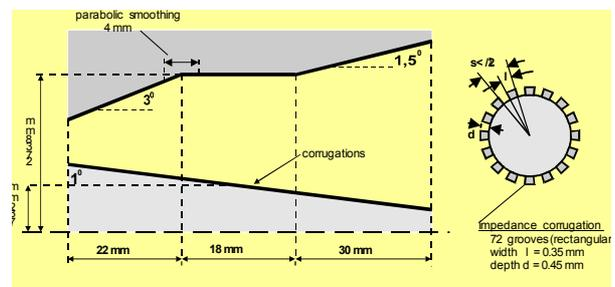
Figure 5. Geometry of the  $TE_{34,19}$  coaxial cavity.
