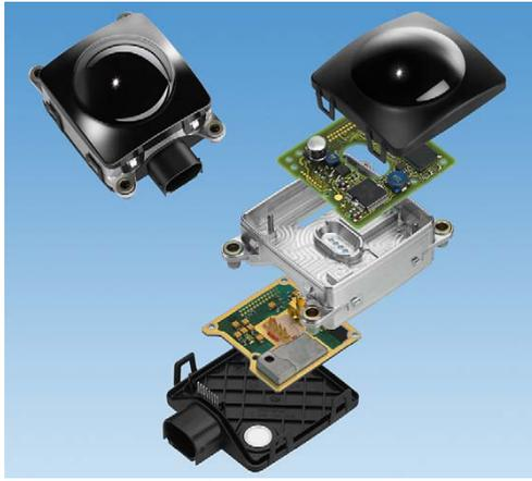
Fig. 1. Bosch ACC, 2<sup>nd</sup> generation
