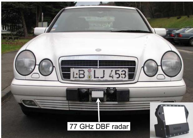
Fig. 6. Test vehicle with 77 GHz DBF demonstrator (also insert in right bottom corner)
